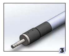
INSULATION IS COMPLETED WITH HEAT SHRINK TUBE
